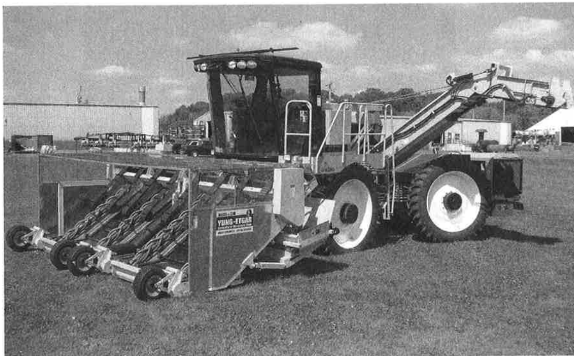
Fig. 17.9. Yung-Etgar/Oxbo Harvester for four rows of dry or fresh chilli (Oxbo Corp.).
