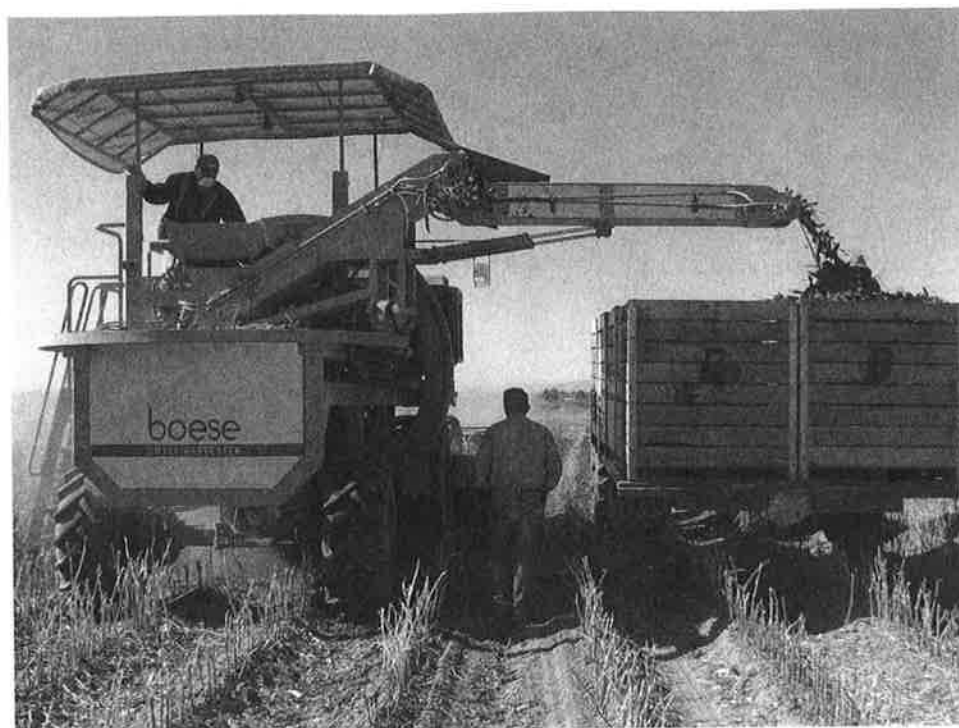
Fig. 17.4. Boese Harvester picking four rows of dry red chilli near Hatch, New Mexico.
