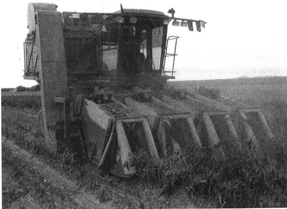
Fig. 17.6. McClendon Harvester picking four rows of dry red chilli near Hatch, New Mexico.
