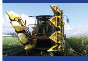
The corn harvesting head, which conveniently folds up for road transport, is designed for easy operation and maintenance.
