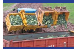
The unique broccoli dump forklift is an integral part of the vehicle, eliminating the need for an additional tractor and operator when pouring the produce into large containers.
